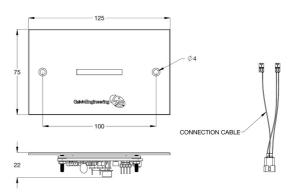
The Galvin Flowmatic<sup>®</sup> Stainless Steel Plate with Concealed 24V AC Wall Sensor to suit Enw. is an aesthetically pleasing, single temperature water control unit, which can be used in hand basins, sinks application to initiate a controlled flow of water.
