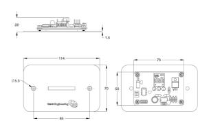
The Galvin Flowmatic<sup>®</sup> Stainless Steel Plate with Concealed 24V AC Wall Sensor for TZFLOWTAPC24 is an aesthetically pleasing, single temperature water control unit, which can be used in hand basins, sinks application to initiate a controlled flow of water.
